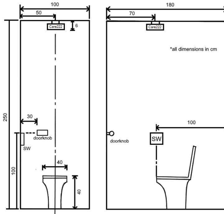
Figure 9: Dimensions of experimental setup in bathroom stall
