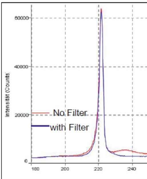
Figure 2: Spectral graph of Excimer lamp with and without short pass filter
